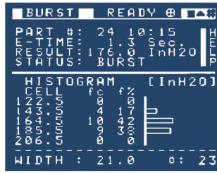
Accumulating test data are shown in histogram form to give a visual overview of your process.
