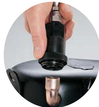
Sealing of expanded tubing for testing and filling applications.
